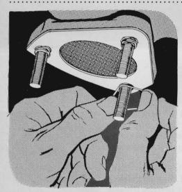
A manifold exhaust-pipe gasket can be held in place on the exhaust-pipe flange, when you're installing the head with manifold attached, by slipping rubber bands over the studs below the gasket. You don't have to remove the rubber bands before tightening the connection.
