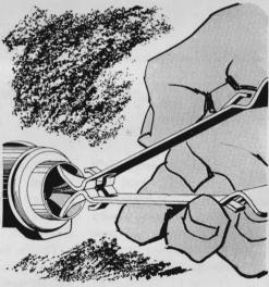
Removing the pistons from hydraulic-brake cylinders for repair can be a tough job. Here's a simple way to do it: Put two puncture-type beer-can openers back to back. Poke their points inside the cylinder so that they bite into the the piston inner lips, and pull.
