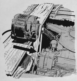
An emergency battery charger can be easily improvised if you have a bench saw with a separate motor and a spare belt. Run the belt from the motor to the alternator (or generator), start motor and run for 15 minutes. This should recharge your battery enough to start the engine.
