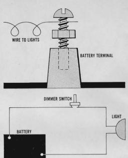
Need a remedy for loss of headlights? Drill a small hole in the center of each battery terminal, insert stainless-steel screws, and wire them via a dimmer switch to auxiliary lights, bypassing all normal circuits. Be sure that you ground the new wiring independently.
