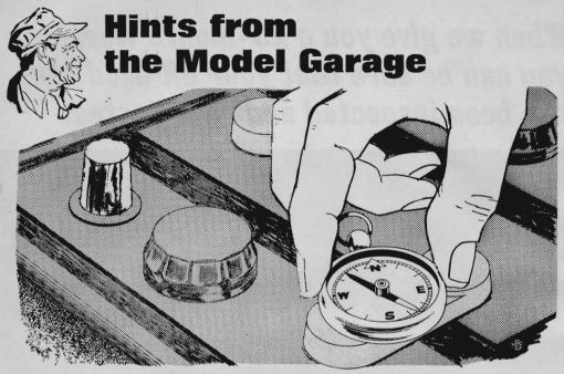
If you should drop the battery when lifting it from your car, or have other reason to believe that there's an electrical leak between the battery cells, you can use an ordinary compass to make a check. Here's how: Set the compass on one of the connectors between the cells. If the needle
