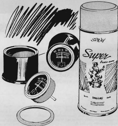
Want additional gauges? Many car owners do — and many have difficulty getting housings. The caps from spray cans (plastic or metal) will serve fine. If you don't want to cut new holes in the dash, mount extra gauges under the dash and in the hole left by a discarded clock.
