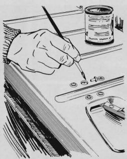
A drop of shellac or varnish on the hole will prevent damage to fresh paint when you reattach moldings or accessories. The shellac will keep the screwhead from cracking the paint and opening the way for moisture and rust formation.
