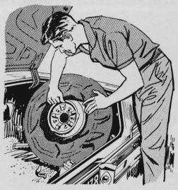
Avoid the dirt of flat tires by keeping the spare in a cover made from an oversize inner tube, washed with soap and water, with valve stem removed. When a tire goes flat, snap the cover on before removing the wheel, and then change wheels.
