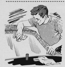
To clean plastic windows on convertibles, use some jeweler's rouge on a wet cloth. Apply the paste with even strokes, up and down, and wipe dry with a clean piece of cloth. The same treatment works on the plastic of portable radios and TV faces.
