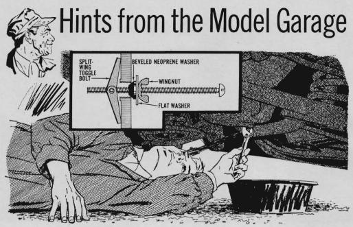
Thread gone in your oil-pan plug hole? You could bore it out and tap for an over-size plug but such plugs are rarely available, and a full repair job, involving removal of the oil pan, welding in of a new nut assembly, and reassembly, would come
