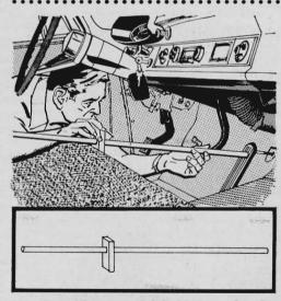
An adjustable gas-pedal hold-down, handy when checking the engine (or warming up), is easy to make. You need a %-by-32" hardwood dowel and a %-by-2"-by-5" block. Drill the hole in the block  $\frac{1}{32}$ " larger than the diameter of the dowel.
