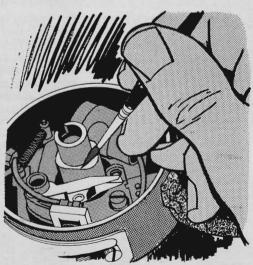
Relocating a distributor shaft after removal may be a problem. To help you replace the distributor on the correct lobe, you can dab a drop of paint, before dismantling, on top of the lobe at the spot where the rubbing block hits the lobe.
