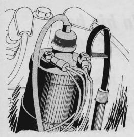
A mysterious engine miss can be traced to the dipstick on some late-model Studebakers and other cars. If the stick is not completely pushed home and the loop of the handle is by mischance turned the wrong way, it can short out the coil primary wire.
