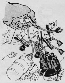
Distributor-lead order can easily be mixed up when replacing wires in a V-8 distributor cap or replacing the cap. Eight numbered spring-type clothespins make it easy to keep track of which wire goes where if you have to remove them all at once.
