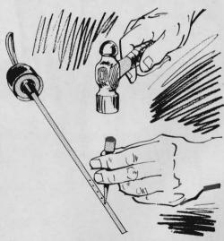
Reading oil level with clean oil on the dipstick often can be difficult. Make it easy by prick-punching a series of dents in the dipstick. Oil will collect in the punch marks and show the level clearly. Small drilled holes work even better for visibility.
