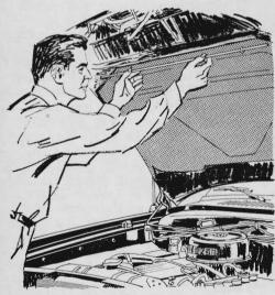
A loose insulation blanket under the hood can cause trouble. Fasten it with a thin rod across the front blanket edge, using a wire hook at each end. If the blanket is already damaged, protect the air-cleaner intake by adding a piece of screen wire.
