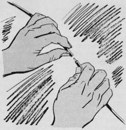
A broken or cracked windshield washer line can be fixed by snipping off a piece of ball-point pen refill, inserting it into the broken line, joining the pieces and taping them. The refill is plastic, and a half-inch can be cut with no damage to the pen.
