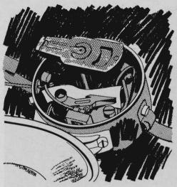
To check distributor points the fast way, insert a piece of paper stapled to a piece of carbon paper between the cam and the rubbing block. Turn the engine with the starter and check carbon imprint. If full contact is not shown, straighten the rocker arm.
