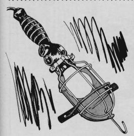
Most trouble lamps will roll if placed where they light up the spot where light is most needed. Stopping the rolling is easy: Just bore two holes in a metal strip 6" long and secure it to the lamp with a thin spring around the light guard.
