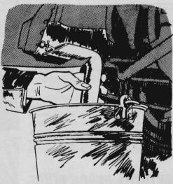
When you drain your radiator, you may lose precious antifreeze because of the drain-cock position, which causes dripping and splattering. Save the fluid by making a diagonal cut in an old elbow water hose and draining through it into a bucket.
