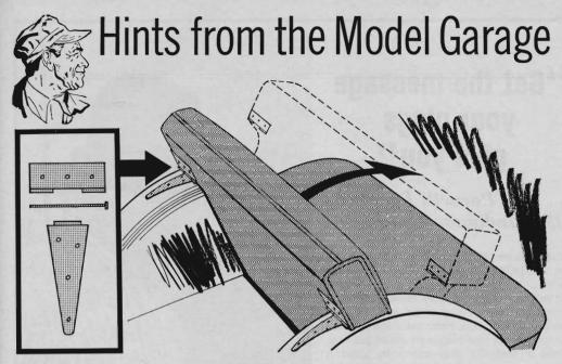
Securing the side latches on the secondseat folding backrest is a matter of concern to many station-wagon owners. During hard braking, heavy loads pushing on the backrest may force the standard latch to give so that the second seat collapses. To accommodate long objects, it must still be possible to fold the backrest. The solution: barn-door hinges, installed as shown. Pull out the pins, and you can fold the backrest forward; when the pins are in position, the seat is completely secure.
