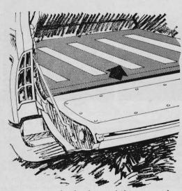
To prevent loads from shifting on the smooth metal rear deck of a station wagon, apply strips of adhesive-backed antiskid tape. This material is sold in hardware stores to provide an antiskid surface in bathtubs and on stone steps.
