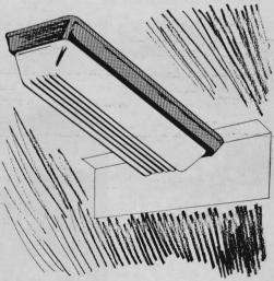
A car's dome light can be used at night by back-seat passengers without disturbing the driver, if you install a cardboard shield. Wedge the bent edge between the light and the headliner. Position it so it casts a shadow over the driver's area.
