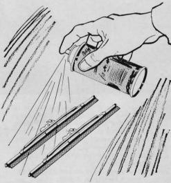
Keep windshield-wiper blades "alive" longer by coating them with silicon slick spray from an aerosol can. The slippery coating reduces friction between blade and windshield, prolonging blade life and greatly improving their water-wiping efficiency.
