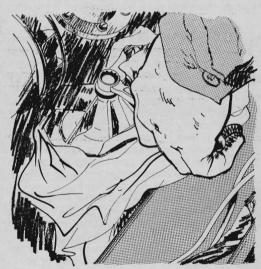
Changing an oil filter won't be such a dirty chore if you wrap a plastic bag around the filter housing before removing the retaining bolt. The same trick works with spin-off filters: Slip the bag over the filter before fitting the strap wrench.
