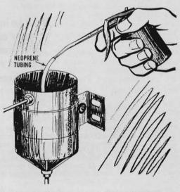
When replacing an oil filter, the housing can be pumped dry of dirty oil with an oil-can fitted with a short length of neoprene tubing as a nozzle extension, as shown above. Wipe out whatever drops of dirty oil remain in the housing with a rag.
