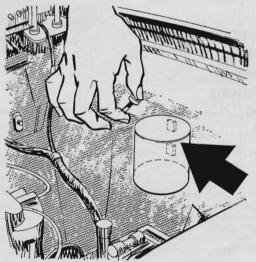
You won't lose small parts (nuts, bolts, washers) if you try this idea: Solder two magnets to a small can. The magnetized can will then stick to the cowl, hood, or other convenient places while you work. Keep the parts in the can until needed.
