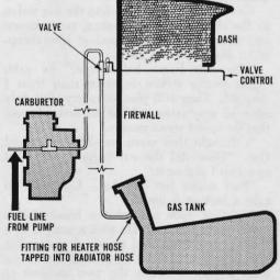
Vapor lock can be cured by a bleed valve and new pipe leading back to the gas tank. Couple the pipe to the fuel line with a T union. Mount the valve on the firewall with linkage to a handle under the dash. Open the valve whenever vapor lock threatens.
