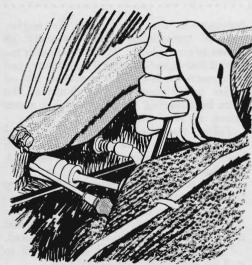
Stuck spark plugs can be removed intact from V-8 engines with deep wells if you place a small-handled %" screwdriver alongside the socket extension in the well. This way, all necessary force may be used on the handle without breaking the plug.
