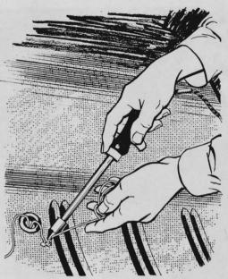
If a gas gauge gives erratic readings in any 1957 or later Chrysler car, it's a safe bet that the tank unit has a poor ground connection. A simple remedy: Solder a wire from the twist-on plate to some nearby spot on the body shell of the automobile.
