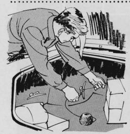
Loose packages in the trunk won't rattle around if you tie them down by means of marine cleats on the trunk walls. Fasten the cleats with self-threading metal screws. Ordinary twine will hold the packages. Marine-hardware stores carry the cleats.
