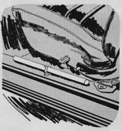
Keep your road flare handy for an emergency by fitting a broom-closet clip on the door sill next to the driving seat, as shown above. One clip is usually enough to hold the flare in place, but two may be used if there is enough space for them.
