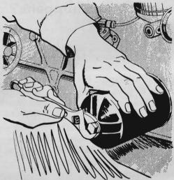
When installing an oil-filter element in a top-cover or shell-type casing, be sure to hold the cover or shell tightly in place while tightening the center bolt. If you keep the shell from turning, the gasket will seal and assure freedom from leaks.
