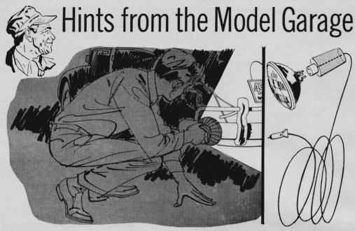
A low-cost trouble light is easy to make from an old auto head lamp. It doesn't matter if the low beam is burned out, but the high beam must be okay. Remove the plug end from a 20-foot extension cord, thread the cord through a hole (punched
