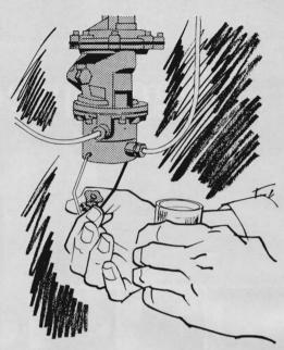
On cars with sediment bowls at the bottom of the fuel pump, the easy way to disconnect the fuel line on the pressure side of the pump is to remove the bowl. In this way, the engine can be turned over without risk of gasoline running all around.
