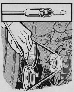
Chalking those hard-to-reach marks on the crankshaft pulley and index pointer can be a lot easier with a chalk holder made from a discarded radio antenna. Cut 2" slots in the hollow tube and flare it to fit the chalk. Rubber bands hold it tight.
