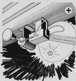
Keep forgetting to push the choke knob back after the engine warms up? A warning light is an ideal answer. It can be made from a low-cost clamp-on running lamp and a mercury switch. Wire the lamp and switch in series to the accessory terminal of the ignition switch. Make a shade for the bulb by taping a white card into a cone, with red cellophane covering a hole.
