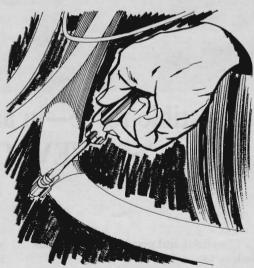
To prevent kinks from forming at sharp bends in radiator or heater hoses, place a worm-drive type of hose clamp at the middle of the bend. Tightening the clamp until it grips firmly will force the hose into a correct cross section and permit the full flow of coolant. In addition, the hose is less likely to leak when there are no kinks in it to weaken the rubber.
