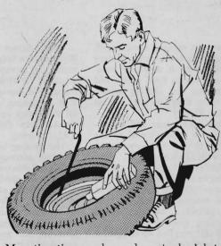
Mounting tires can be made easier by lubricating the beads before you start to lever them over the edges of the wheel rims. A squirt or two from a handy squeeze bottle of any liquid soap (not detergent) will work wonders for you as a labor saver.
