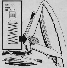
When the horn contact on '59-60 Thunderbirds becomes badly worn, a permanent fix can be made by cutting the tip off a metal tire-valve cap, and removing the rubber insert. Smooth off the cut and slip the cap over the contact-spring end to extend it. More Hints from the Model Garage
