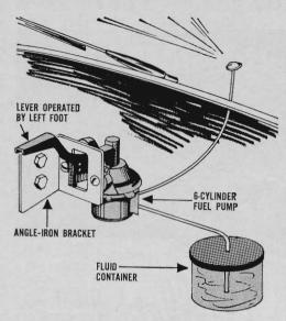
Make your own windshield washer by mounting a fluid container on the firewall or on the engine-compartment sheet metal. Run a pipe to a six-cylinder-Ford fuel pump fastened with an angle bracket to the left side of the cowl. Add a foot lever and run tubing to the nozzles.
