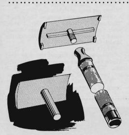
To remove upper halves of main bearings, improvise a tool from an old safety razor. Discard the backing plate and grind away all projections on the faceplate. Cut the handle in two. Turn down the top half in a lathe until it fits the journal's oil hole; then screw it back on (left).
