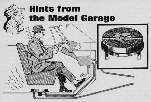
A common fault of under-dash heaters is the lack of heat for rear-seat passengers. Solution: Install an under-seat heater (from any 1948-1955 General Motors car) under the front seat, discard the heater cover, and cut holes in the floor for the fan motor and hose connections.
