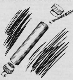
To store spare valves so they won't stray or get damaged, carry them in a container that's also a tool for removing and replacing tire-valve cores. Solder a valve cap on a short piece of %" brass or copper tubing. Close the other end with a tight-fitting plastic cap.
