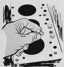
Keep dirt and carbon out of the lifters by plugging up the pushrod holes whenever you're grinding the valves or decarbonizing the cylinder head. Ordinary medicine-bottle corks can easily be made to fit. Leave them in the holes until reassembly.
