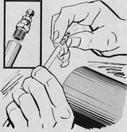
A leak in an external oil or brake line can be fixed by removing the line and screwing in Zerk grease fittings borrowed from the car's chassis. This will keep you going without an oil filter, or with three-wheel brakes, to the nearest garage.
