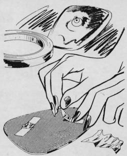
Bare spots on your mirror where the silver has come off can be fixed. Carefully remove the glass and cover the spots on the back of the mirror with tinfoil. Use clear, waterproof, adhesive tape to hold the foil securely, covering the patch completely.
