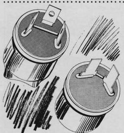
If your flasher unit fails, you can easily make a bypass, using a short wire (or a strip of folded metal foil) to connect the X and L prongs on the base of the unit. Refit the flasher unit in the socket and make flashing signals by switching on and off.
