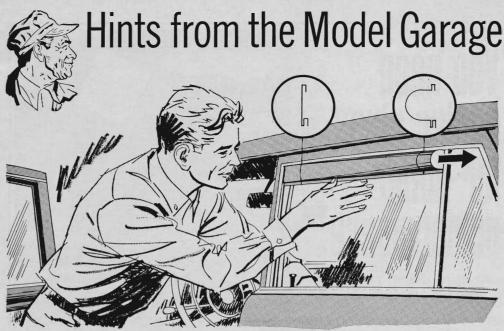
Exhausting air from a car is a problem. You can always get outside air in, but on many cars the only way of letting it out is to open a window. Vent panes are noisy at high speed and also set up drafts that hit the passengers on the opposite side. The
