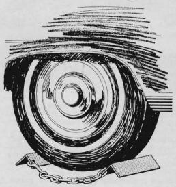
Keep your car from rolling off the jack when you change a tire with this pair of safety wedges. Make them by chaining together two 8" lengths of 1½" angle iron or tempered-aluminum angle. Place the wedges against the unjacked wheel on the lifted side.
