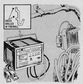
Hang your battery charger on a hook made by mounting a medium-size pegboard hook in your car firewall. Drill two 3/16" holes on 1" centers, and slip the hook in place. Besides being convenient, the charger gets sufficient ventilation to prevent overheating.
