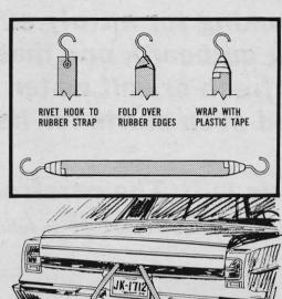
Make a trunk-lid hold-down strap, for use with oversize loads, out of a rubber strip cut from an old inner tube. Rivet a steel hook to each end, and finish as shown above. Hint: Make up several straps of different sizes so you have one to fit any load.
