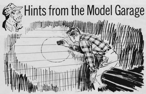
For precise headlight alignment, use a photo exposure meter to find the beam's brightest spot. Set up an aiming target (see your car's service manual), and scan the headlight-beam pattern with the meter. When you locate the hot spot, align the headlight
