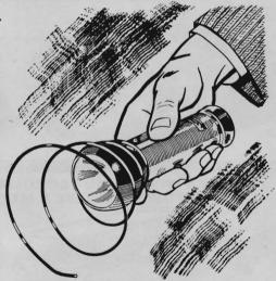
Make your auto flashlight breakproof by wrapping the smaller turns of a cone-shaped furniture spring around the body at the head. This will give the lens the same kind of protection the wire guard gives to the trouble light you use in your garage.
