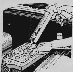
Date it when it's new and you won't forget how old your battery is. Use a sharp point to scribe figures on a cell post or connector, fill them in with white calking compound, and wipe off the excess. The reminder will be legible despite engine grime.
