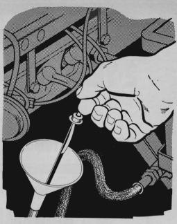
Make a dipstick guide from a polyethylene funnel so you can replace the measuring stick without fumbling. Cut off the funnel at the narrowing end until it can be pushed over the dipstick tube. The flexible plastic's "give" allows a tight force fit.
