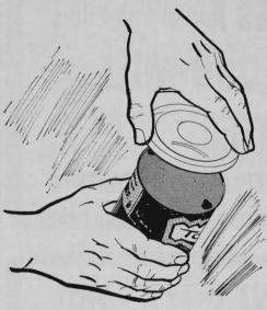
You can safely store cans of partially used motor oil or transmission fluid by slipping a plastic coffee-can cover over the top of the container. The plastic is just the right size for quart cans. It keeps dust out and fits tightly to make the cans spillproof.
