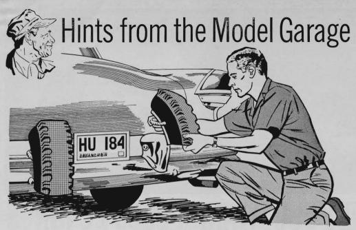
Protect the chrome on your bumper with this simple trick when you have to give or get an emergency push: Drop a pair of rubber cushions made of old tire sections over the bumper guards. Cut the sections from any discarded casing and make a hole on each side, inside the bead. Loop a rope through and knot it on each end. The rope, when slipped over the guards, keeps the cushions from slipping. You can store the cushions in the trunk over your spare tire where they'll always be easy to find.
