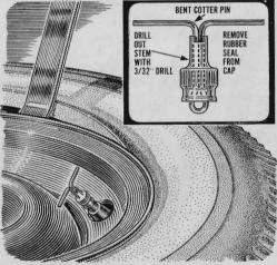
Make an inexpensive holder to retain tiretube valve stems and they won't slip inside the rim when you're mounting a tire. Drill a hole through the end of a standard metal valve cap large enough for a cotter pin. Put in the pin and spread out the legs.
