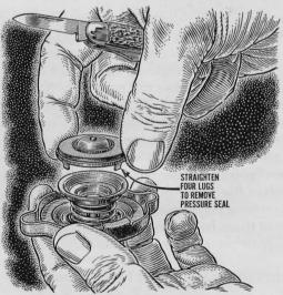
For emergency treatment of a leak in your car's cooling system, unscrew the pressure cap and remove the rubber gasket. This will reduce the pressure 12 to 15 pounds and stop most leaks. Keep the rubber seal -you'll want to replace it after repair.
