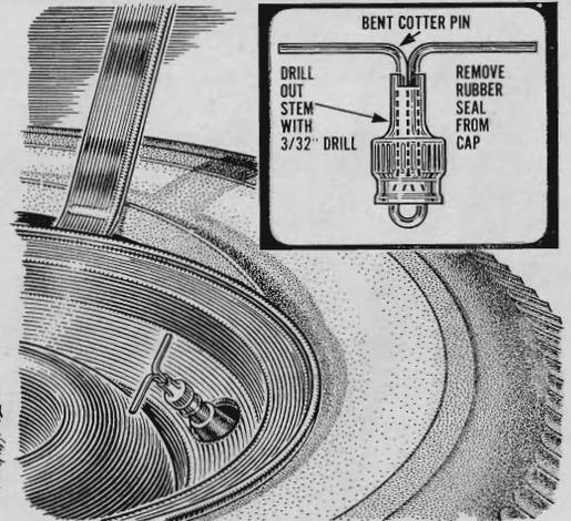
Make an inexpensive holder to retain tire-tube valve stems and they won't slip inside the rim when you're mounting a tire. Drill a hole through the end of a standard metal valve cap large enough for a cotter pin. Put in the pin and spread out the legs.
