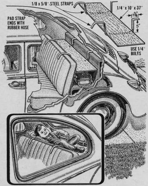
A simple crib for the baby can be made for the luggage compartment behind the back seat of a Volkswagen. All you need are a piece of plywood or hardboard, stove bolts, and 1/8"-by-5/8" steel strap for hangers. For safety, add a baby-carriage harness.
