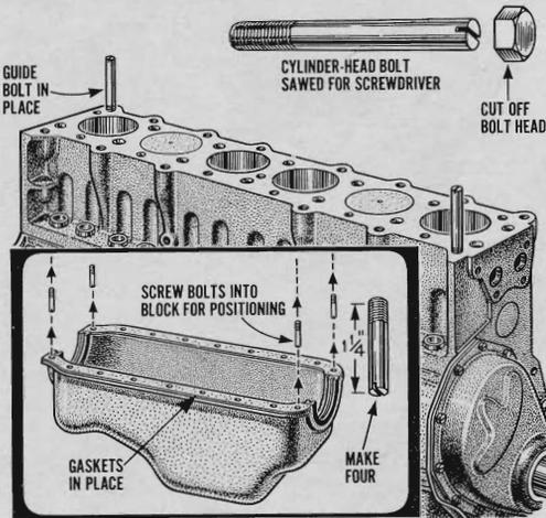
Installing cylinder heads and oil pans of some types can be made easier with guide bolts. Make them by cutting off the tops of old head and pan bolts, and slot them to take a screwdriver. They are easily removed when the head and pan are in.
