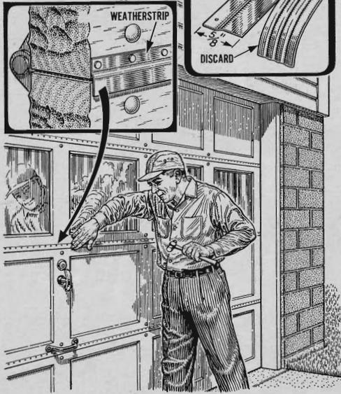
To prevent water accumulating in a horizontally split garage door, snip in half 1 1/4" bronze weatherstripping. Nail the perforated half of the strip to the upper edge of the door at the split, letting it lap over the crack. Paint it the color of the door.
