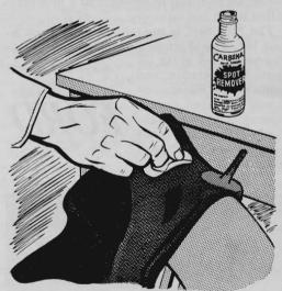
For a long-life inner-tube patch, clean an inch-wide area around the tear with a carbon tetrachloride cleaning fluid (such as Carbona spot remover). The fluid prepares the rubber surface for a patch without the usual preliminary sanding and scraping.
