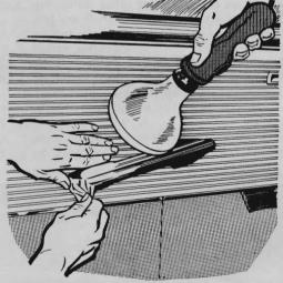
Soften vinyl-plastic upholstery material before covering armrests, by exposing it to an infrared heat lamp for a few minutes. You can easily stretch the softened vinyl around and under the curved ends for a neat, wrinkle-free re-covering job.
