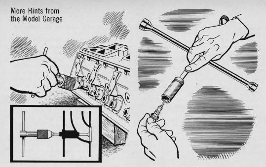
When you're grinding valves and the vacuum cup on the grinding tool won't grip the valve properly, try this. Place the engine head on edge and grip the valve stems with a large-size tap wrench. Turn the handle back and forth, using only a light pull.
