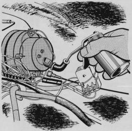
Oil a squealing speedometer this way. Disconnect the cable and press the large end of a rubber spark-plug shield over the connection on the housing. Then insert a pump-type oil can into the shield's small end and squirt in three or four shots.
