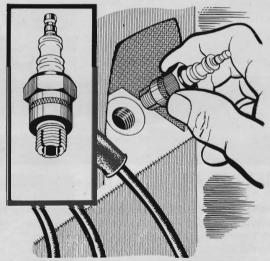
If the threads are spoiled in a spark-plug hole, here's a quick way to restore them without a tap. Hacksaw two cross slots in an old plug and squeeze the sections slightly together in a vise. Then run the plug into the hole to clear the threads.
