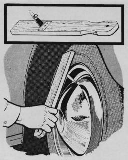
Make a hubcap puller from a 14" length of one-by-three and a strap hinge. Shorten the strap, leaving about 2\mathbb{X}". Bend up the last \mathbb{X}" in a vise to form a hook. Screw the hinge to the board about 5" from the end and cover the hook with adhesive tape.
