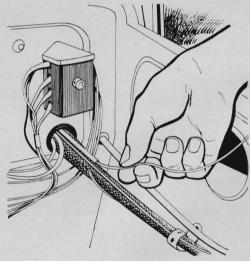
Running an extra wire through a grommet that's already packed with wires can be difficult unless you first insert a short length of metal tubing with an inside diameter larger than the wire. Pass wire through the tubing, then remove the tubing.
