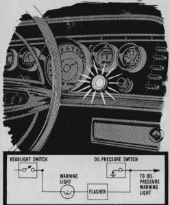
If you forget to turn off your lights, an extra lamp wired in as shown will warn you. With the engine off but the lights on, the warning lamp will light up. With the engine running, ground path to warning light is broken by the oil-pressure switch.
