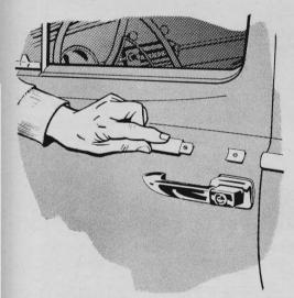
Cut out your own chrome-trim clips from a large tin can. Snip clips the exact width of molding, drill holes in their centers, and attach them to the car with metal screws. The curve of the can flares the clips out, making it easy to slide trim on them.
