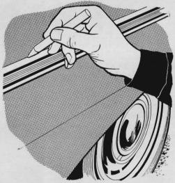
Prevent rusting around chrome trim by sealing the crack between the trim and the body metal. Put a point on a stick of lubricant and apply the lube along the length of the trim. This will keep water from getting down inside the molding.
