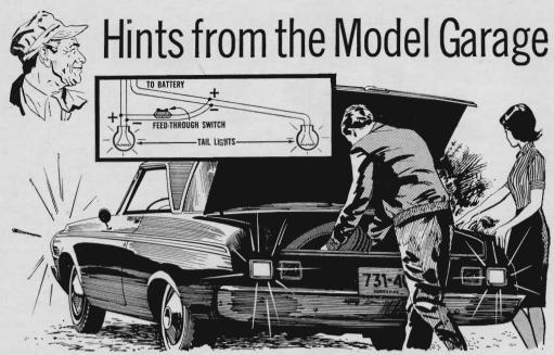
With all four blinkers flashing, you don't need flares when you stop at night for repairs. Connect both tail lights with two insulated wires. On one wire, connect a feed-through switch. In an emergency, turn on the switch and the turn signals. To
