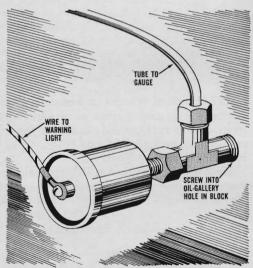
When installing an oil-pressure gauge in a car equipped with only a warning light, use a brass T fitting so the gauge and light both work. It's a good idea to retain the light; it will draw your attention faster than the gauge if pressure drops suddenly.
