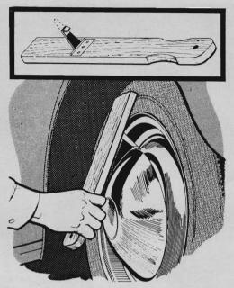
Make a hubcap puller from a 14" length of one-by-three and a strap hinge. Shorten the strap, leaving about 2\mathbb{\pi}". Bend up the last \mathbb{\pi}" in a vise to form a hook. Screw the hinge to the board about 5" from the end and cover the hook with adhesive tape.
