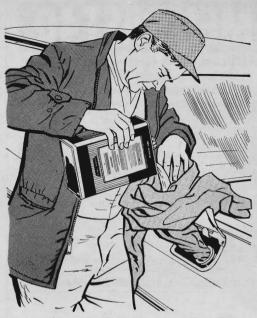
When you run out of gas along the road and there's no funnel handy, use a plastic raincoat to pour gas into the tank without spilling. Stuff a sleeve into the filler neck; pour gas into the armhole. Rinse the coat in water to remove the smell of gas.
