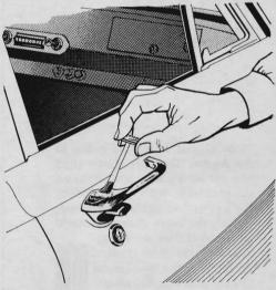
When you paint a car, some places are almost impossible to cover with masking tape. To protect these inaccessible spots, simply brush on some rubber cement. After the painting's done, you can easily rub off the cement—along with the overspray.
