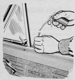
Lubricating window-lift gears is easy if you make a tiny funnel for the oil. Cut off a small piece of copper tubing and flare one end. Run the window down and push the tubing into the slot until it rests on the gear. Drop oil into the flared end.
