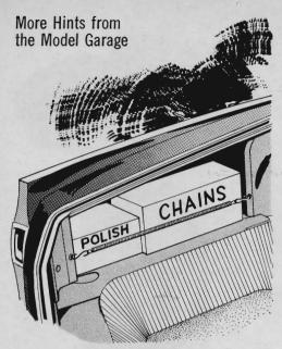
To keep your trunk neat, use a ½" screen-door spring. It'll hold packages, chains, and other items securely in place along the side. Drill holes in the wheel-well metal and tail-light brace, and fasten the stretched screen-door spring with S hooks.
