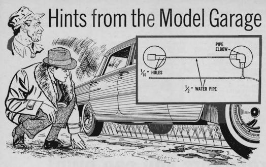
An undercarriage spray washer prevents corrosion from road salt used in icy weather. Make it in a U shape, using two long pieces and one short piece of ½" water pipe, joined with an elbow at one corner and a garden-hose connector at the other.
