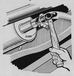
Use a muffler clamp to force a tailpipe into the muffler outlet. Invariably the pipe has to be hammered to get it to seat properly. By fastening a clamp near the end of the pipe that goes into the muffler, you have something to hammer against.
