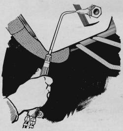
When threads are stripped in the crankcase drain-plug hole after long use and no bolt will tighten properly, get out your welding torch and a nut. Braze the nut securely over the hole, and then plug it with a matching bolt and a washer.
