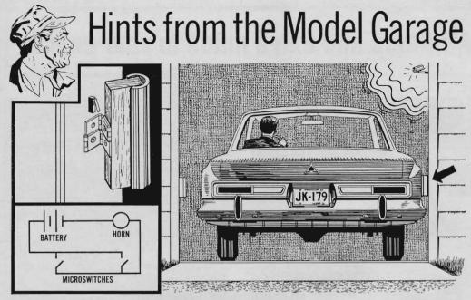
Microswitches can prevent damage to your car when you pull in and out through a tight garage opening. On each side of the opening, at the same level as the widest part of your car, mount a switch behind a wood block secured by a double-acting spring hinge. Cover the edge of each block with a strip of garden hose, and wire the switches to a flashlight battery and a bicycle horn. If your car touches one of the wood blocks as you drive past, a blast from the horn warns that you're too close.
