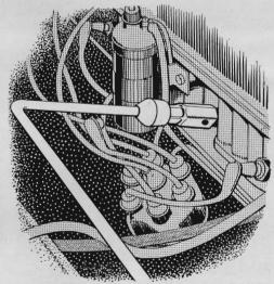
Spark plugs screwed in too tightly are a problem to remove. One reader, having bent his plug wrench in trying to force removal of a hard-to-get-out plug, found that his wheel-lug wrench socket fit the plugwrench hex. The plug came out easily.
