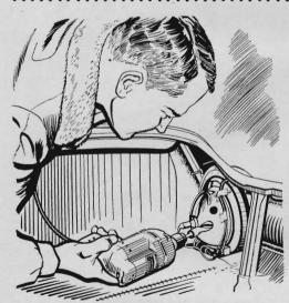
Need a handy trunk light for emergencies after dark? Simple: Drill two ¾" holes in each tail-light housing where it protrudes into the trunk. Then, when you turn on your parking lights, more than enough light will spill over into the trunk.
