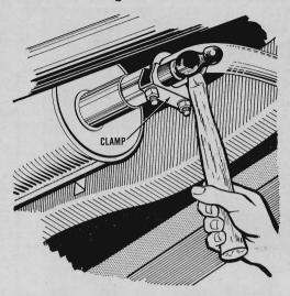
Use a muffler clamp to force a tailpipe into the muffler outlet. Invariably the pipe has to be hammered to get it to seat properly. By fastening a clamp near the end of the pipe that goes into the muffler, you have something to hammer against.
