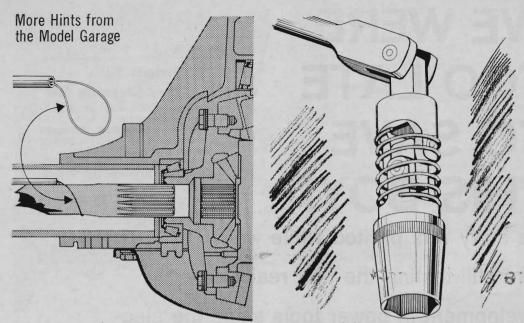
Pieces of a broken axle can be removed with a snare without taking off the differential cover. Slip a flexible wire, looped on the end, through a piece of tubing. Insert in the housing. Move it around to locate the broken part, tighten the wire, and pull.
