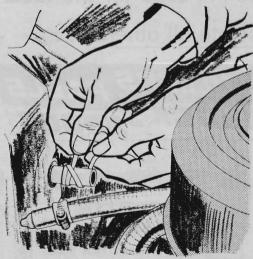
A leaking heater hose can often be fixed with a broad, sturdy rubber band. Disconnect the hose. Wrap the heater pipe connection tightly with the rubber band, spacing the turns evenly under the half-inch area occupied by the hose clamp.
