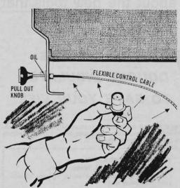
To lubricate sticking flexible cables on dash controls, pull out the knob and apply oil where the wire enters the dash fitting. Heat the cable behind the dash with the cigarette lighter. Oil will be attracted to the heated portions of the cable.
