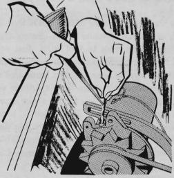
To keep from over-oiling a generator with the customary squirt can, introduce the point of a nail into the spring-covered oil tubes. Let the spring cap hold the nail in place. Then let one or more drops of oil run down the side of the nail.
