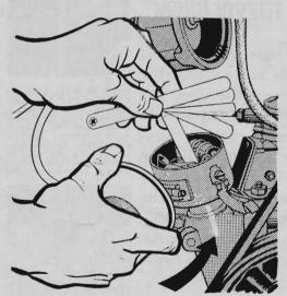
When adjusting point gap, it's easier to position the rubbing block on the cam lobe by turning the distributor. Mark the distributor base. Loosen locking bolt, rotate distributor until gap is maximum. Adjust points, return distributor to mark, and lock.
