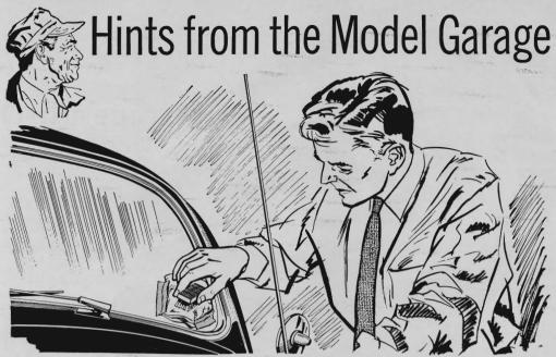
Removing decals from car windows and bumpers needn't involve tedious and messy scraping with razor blade. Just fold a kitchen paper towel into a patch slightly larger than the decal. Tape it over the decal and saturate with household ammonia, using a small brush. Press the paper down occasionally to insure full contact, and apply more ammonia when the paper begins to dry. After about a half hour the decal will dissolve. It can then be wiped off with a damp paper towel.
