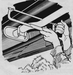
When a muffler must be cut loose, saw the exhaust pipe the easy way. Remove the blade from the hacksaw frame and replace it upside down, with teeth pointing toward the handle. By cutting from the top down, you get more leverage and less binding.
