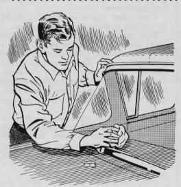
Windshield scratches seemingly made by worn wiper blades may actually be caused by excess windshield sealer oozing from the bottom molding. Wipers pick up this abrasive, cause streaking. Remove smeared sealer with a razor; wash with solvent.
