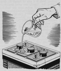
Asphalt-topped batteries last longer if protected with a thin layer of paraffin wax. Wash the battery top and build a cardboard dam around it; a string holds the cardboard. Pour %" of wax over the top to seal cracks that often form there.
