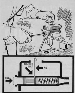
In rebuilding some master brake cylinders, it's easy to install the piston stop and ring by pushing the piston into the cylinder until it passes the breather hole. A pin in the hole holds the piston out of the way while you install the piston stop and ring.
