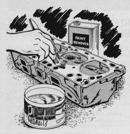
Removing an old gasket during an engine overhaul can be a chore. Instead of wasting time with a scraper, liberally brush on some paint remover. Allow a few minutes for the paint remover to soak in. You'll find that the gasket peels off easily.
