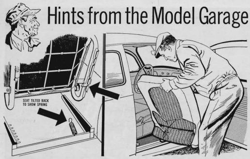
A worn-out driver's seat needn't be a problem in a Volkswagen or in most other bucket-seat-equipped cars. Merely switch driver's and passenger's seats to equalize the wear. On the Volkswagen all you need to make the swap is a screwdriver. Disconnect the retaining spring under the seat, pull the seat forward, and take it off the track. Some foreign sedans require no tools at all. In many sports roadsters, seat backs are secured by nuts, which are easily loosened with a wrench.
