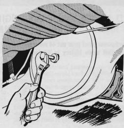
A recessed rear-axle plug can be unscrewed even when the inside corners have been stripped. Drive a bolt into the recess and weld it to the plug. Twisting the bolt with a wrench loosens the plug, allows it to be retightened for further use.
