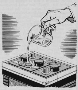
Asphalt-topped batteries last longer if protected with a thin layer of paraffin wax. Wash the battery top and build a cardboard dam around it; a string holds the cardboard. Pour ½" of wax over the top to seal cracks that often form there.
