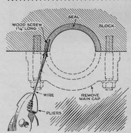
To free a rear main-bearing seal, first remove the bearing cap and drive a wood screw diagonally into the side of the seal, as shown. Then wind a wire around the screwhead and pull the seal out with pliers. The screw provides an anchor to pull on.
