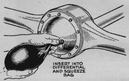
When the differential needs work, you may want to save the grease to replace later. Using a plastic bag makes the job easy. Give the top of the bag a twist to store the grease until your work is finished. Then squeeze the grease back in, as shown.
