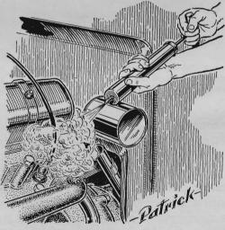
To clean a car engine with degreaser solution, try applying it with a pump-type insecticide sprayer. The spray coats the engine with a fine, clinging film that gets into hard-to-reach crevices. It also saves waste from excessive dripping and runoff.
