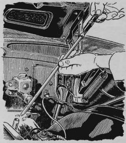
Light up the opening for your oil dipstick by taping a small penlight to the top of the stick. Then spot the opening with a few dabs of luminous paint. You'll not only save time and trouble finding the hole, but you'll have a spare flashlight handy.
